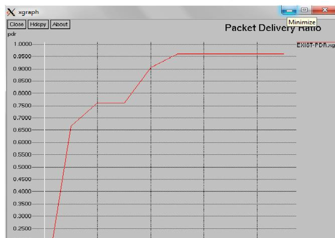
Figure 2.The Graph explains the ratio between the no of packets send and received during the network life.
